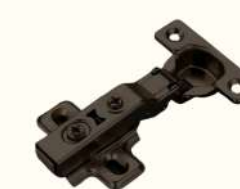
KAH - 12 26mm CUP HINGE (Soft Close) Crank : 0°, 8°, 16° Finish : Black matt
